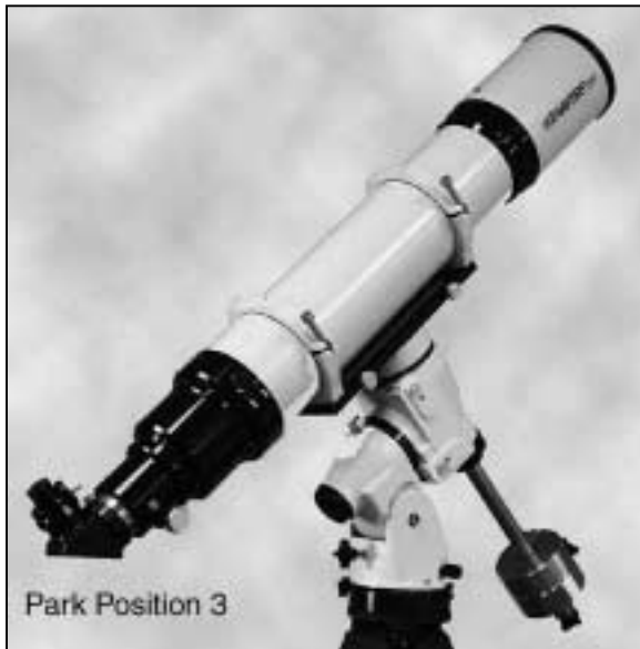
Scope is pointing to the pole. RA axis vertical, Dec = 90
