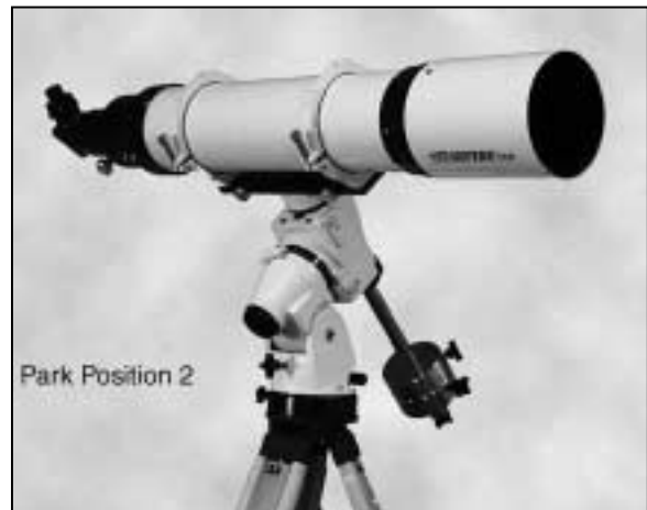
Scope is level and pointing east, RA axis vertical, Dec = 0
